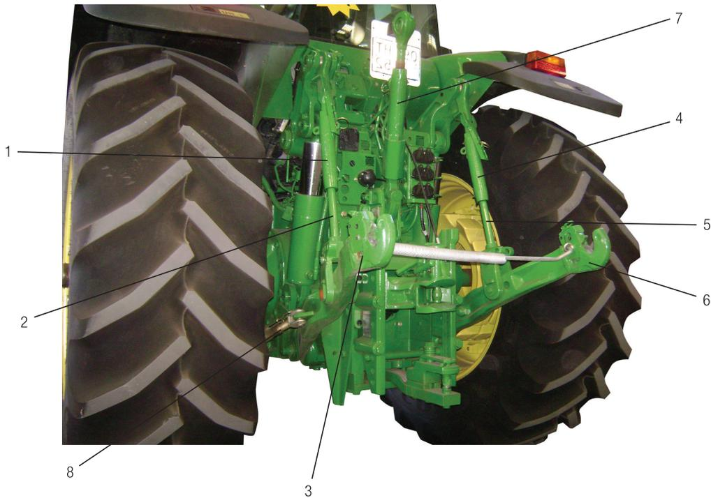
1. Left lower link arm height adjustment mechanism
